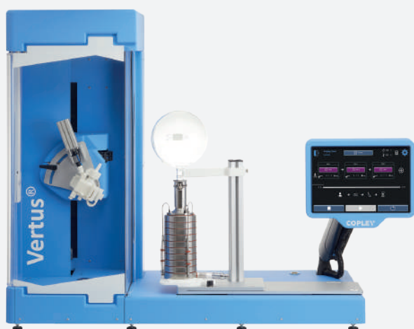
An example test set-up for nasal aerosols.
