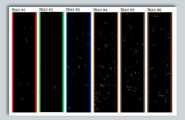
This process can be done with cumulative or non-cumulative measurements. With the cumulative measurement, broken fibers stay in the trays and accumulate over consecutive inspections. With the non-cumulative measurement, the system require the user to clean the trays after each inspection, but it improves the precision, decrease the need for additional manual analysis.
