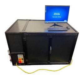
The enclosure is locked during the measurement process for additional safety.
