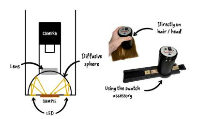
The MAMBO takes advantage of its specific geometry – a diffusive sphere and a stable LED illumination - to always take color measurements in the same and repeatable conditions. Moreover, the color calibrated 12-bit camera enables a high precision comparison of the color of the hair fibers measured and those in its databases without any subjectivity.
