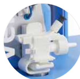
Automated shot weight measurement via an integrated balance
