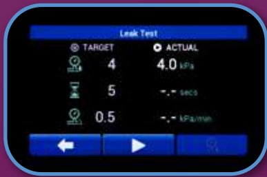
Leak test screen
